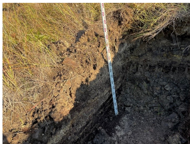
TP12 was excavated about 20m downslope of TP11 and encountered colluvial soil overlying tuffaceous material overlying interbedded claystone/coal followed by practical refusal at 1.3m.
