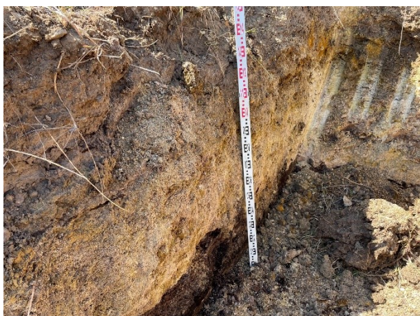
TP6 was excavated in the mid slope of the spur above the access track and encountered a low strength coal layer followed by practical refusal at 1.6m
