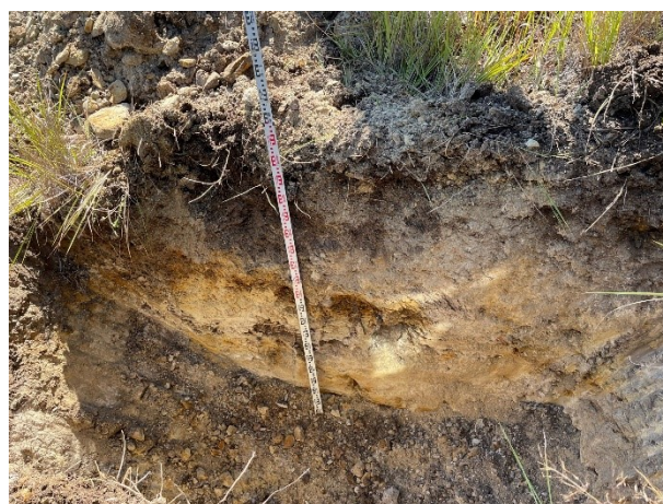
TP 4 was excavated about 20m downslope of TP3 and did not encounter coal seams. The test pit encountered practical refusal at 1.9m
